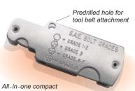
All-in-one compact unit includes bolt sizing blades from 1/4" to 1" SAE sizes and 5mm to 24mm for Metric sizes and full set of common pitch gages.
